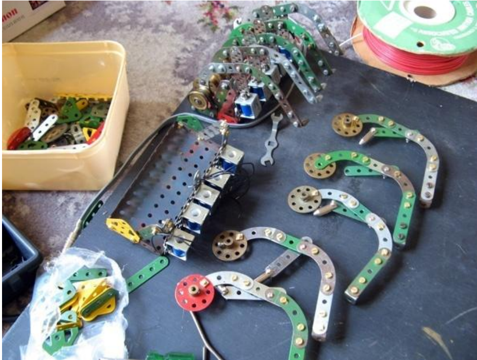
Figure 32: Construction of the Meccano fingers of Fifi, the keyboard player (reprinted with permission from Greg Locke, 2007).
