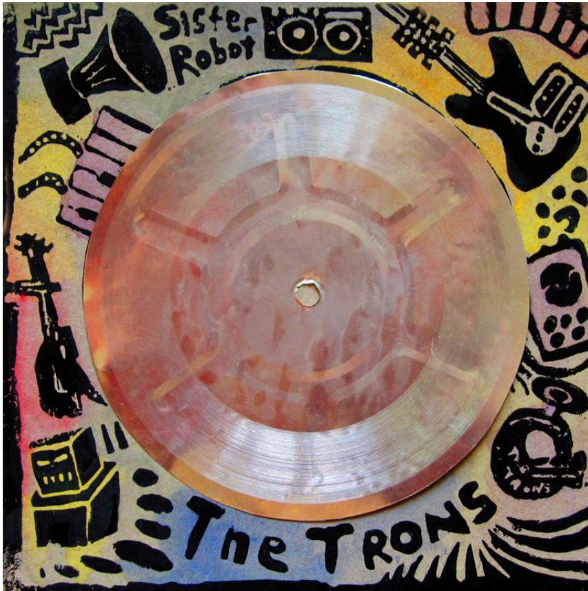
Figure 28: Lathe-cut record of 'Sister Robot' using a discarded aluminium pie-dish (adapted with permission from Greg Locke, 2008).
